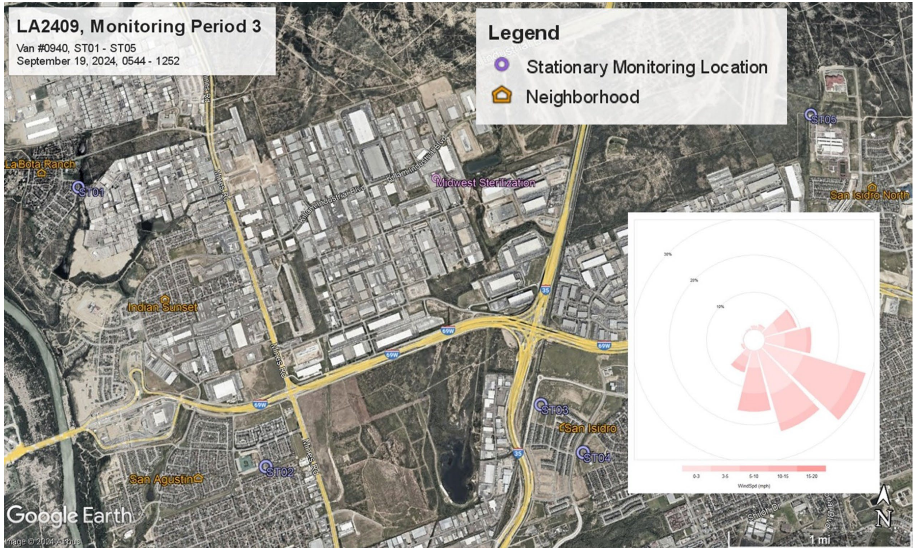
Figure 7: Map of Van #0940 ST01 through ST05 stationary monitoring runs with combined wind rose on September 19, 2024, in Laredo, Texas. All 12-minute cycle ethylene oxide concentrations were below the limit of quantitation of 0.20 parts per billion by volume (ppbv), and all 1-hour average ethylene oxide concentrations were below the limit of detection of 0.08 ppbv. This map was generated by the Air Monitoring Division of the Texas Commission on Environmental Quality. This product is for informational purposes and may not have been prepared for or be suitable for legal, engineering, or surveying purposes. It does not represent an on-the-ground survey and represents only the approximate relative location of property boundaries. For more information concerning this map, contact the Air Monitoring Division at 512-239-1716.
