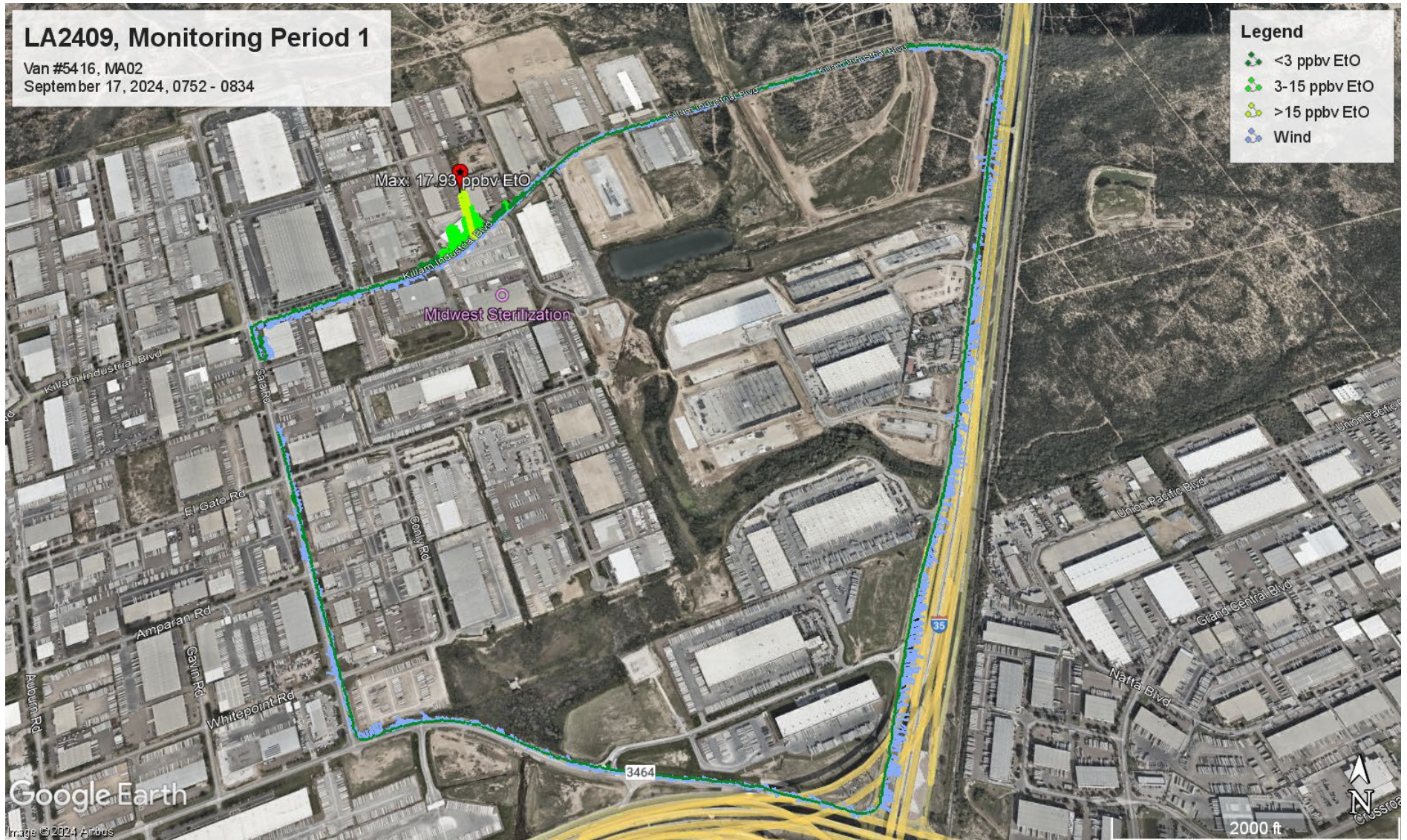
Figure 3: Van #5416 MA02 survey full view on September 17, 2024, in Laredo, Texas. Maximum ethylene oxide concentration of 17.93 parts per billion by volume (ppbv) measured on Killam Industrial Boulevard just north of Midwest Sterilization. Ethylene oxide concentrations east, south, and west of Midwest Sterilization were less than the 3 ppbv limit of quantitation. This map was generated by the Air Monitoring Division of the Texas Commission on Environmental Quality. This product is for informational purposes and may not have been prepared for or be suitable for legal, engineering, or surveying purposes. It does not represent an on-the-ground survey and represents only the approximate relative location of property boundaries. For more information concerning this map, contact the Air Monitoring Division at 512-239-1716.
